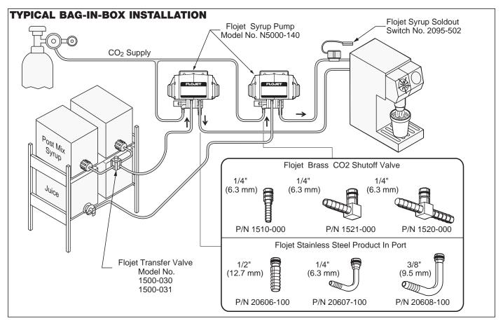
The above diagram shows a "typical bag-in-box installation" with a single bag connection and multiple bag connection with the FLOJET Transfer Valve assembly.
