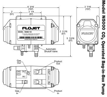
Product "OUT", use reinforced 1/2" (12.7 mm), 3/8" (9.5 mm) or 1/4" (6.3 mm) I.D. hose for discharge. Connect to product "OUT" port and dispensing head product (syrup) connection and clamp both ends securely.
