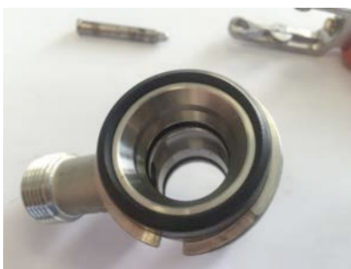
Step 5 : The last seal to change on the S-type keg coupler is the main gasket on the bottom of the coupler. The flat face of the seal is to be located against the body.
