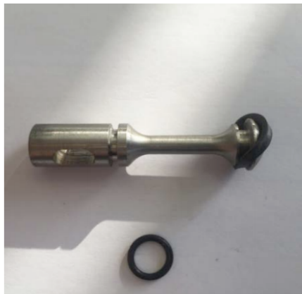
Step 4: Remove shaft o ring from piston and main dome seal & replace
