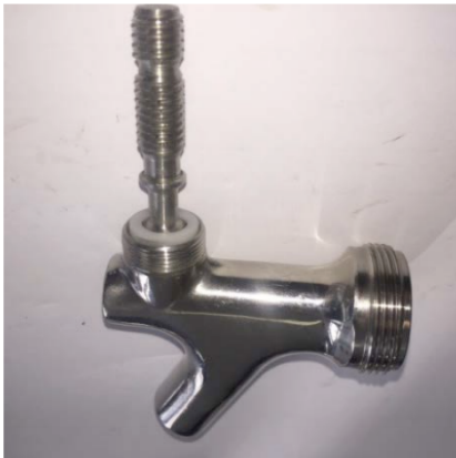
Step 7: Install white nylon friction with depression facing downwards. Install black friction gasket on top and screw bonnet nut clockwise. Tap should move fluidly with light pressure. Firm but free movement.
