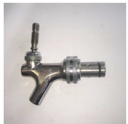
Step 8: Replace coupler gasket and fit shank. Fit coupler nut and gently tighten with C-spanner. Replace shank O-ring.
