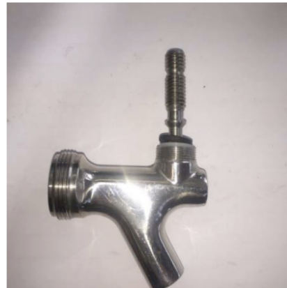
Step 7: Install white nylon friction with depression facing downwards. Install black friction gasket on top and screw bonnet nut clockwise. Tap should move fluidly with light pressure. Firm but free movement.
