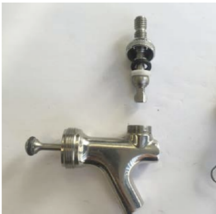
Step 3: Push piston through the body of the tap so that it can be removed from the threaded entrance into the tap.
