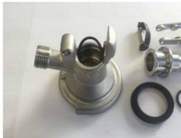
Step 4: There are 2 seals in the body of the keg coupler. Remove these and replace.
